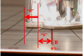
Fig.16 Stylus tip is in front of zero point B.
